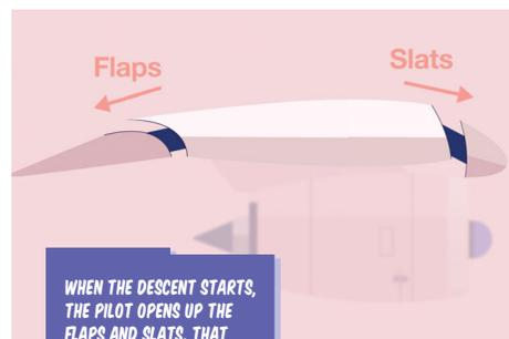
WHEN THE DESCENT STARTS, THE PILOT OPENS UP THE FLAPS AND SLATS. THAT MAKES THE WINGS BIGGER, SO THEY CATCH MORE WIND.
