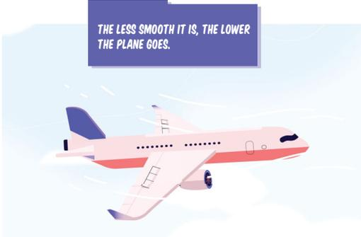
NEXT, THE SPOILERS! THEY'RE LIKE AIR BRAKES THAT MESS UP THE SMOOTH AIRFLOW OVER THE WINGS.
