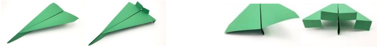
Figure 3: A regular paper plane (left) and a plane with flaps added to the back to increase drag (right) taken from https://cdn.sciencebuddies.org/Files/12708/6/aero-plane-design-cut-flaps.jpg
